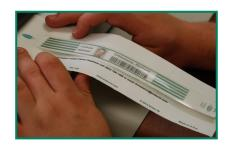
Feed into laminator tab closure end first.
